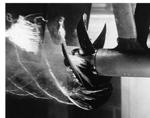
Figure 1 uncontrolled cavitation
